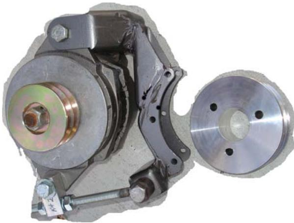
3/4JH4 Forward mount. Specifically for Catamarans or engines with limited forward space. This kit allows easy mounting of a 160 amp Delco or the Balmar 210 amp to fast charge big loads. **\$450USD**
